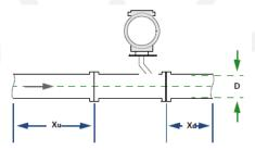
**Image 5.** Installation of In-line Meters (representative)
