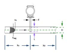
**Image 4.** Installation of Insertion Meters (representative)
